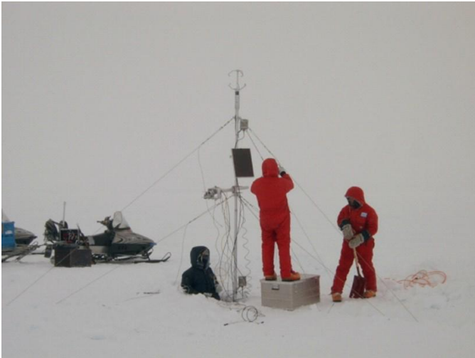
Whiteout during installation of full energy balance AWS at 500 m a.s.l. on NW ramp of Vestfonna (from left: Roman Finkelburg, Dieter Scherer, Christoph Schneider)
