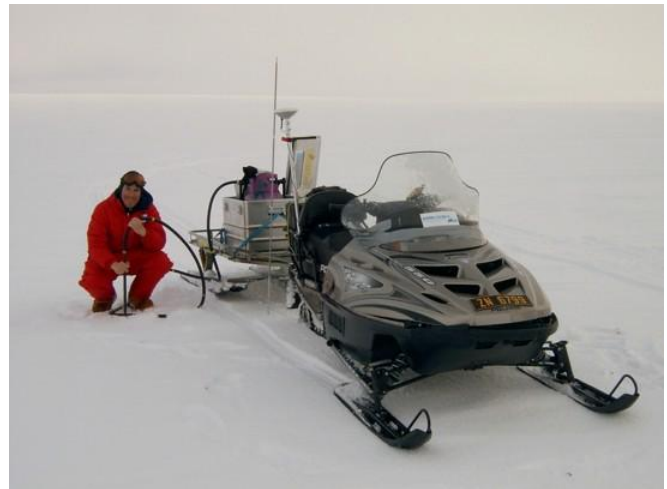
Marco Möller doing steam drilling work for installation of an ablation stake on De Geerfonna
